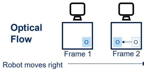
Figure 2-5 Optical flow tracking
