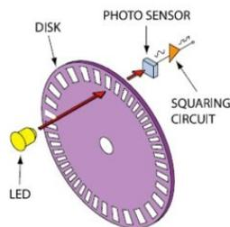
Figure 2-2 Wheel encoder components
