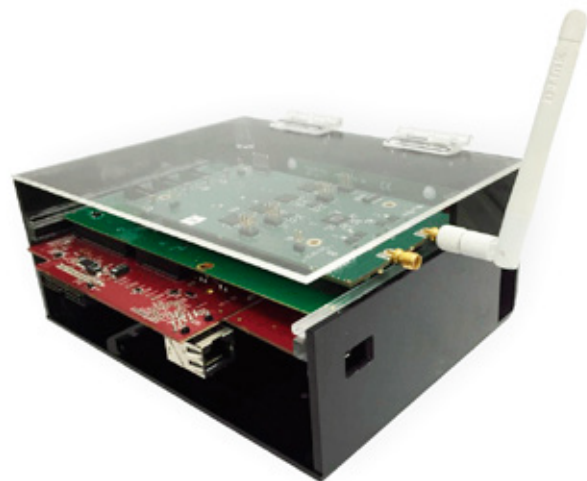
RivieraWaves Wi-Fi IP validation platform
