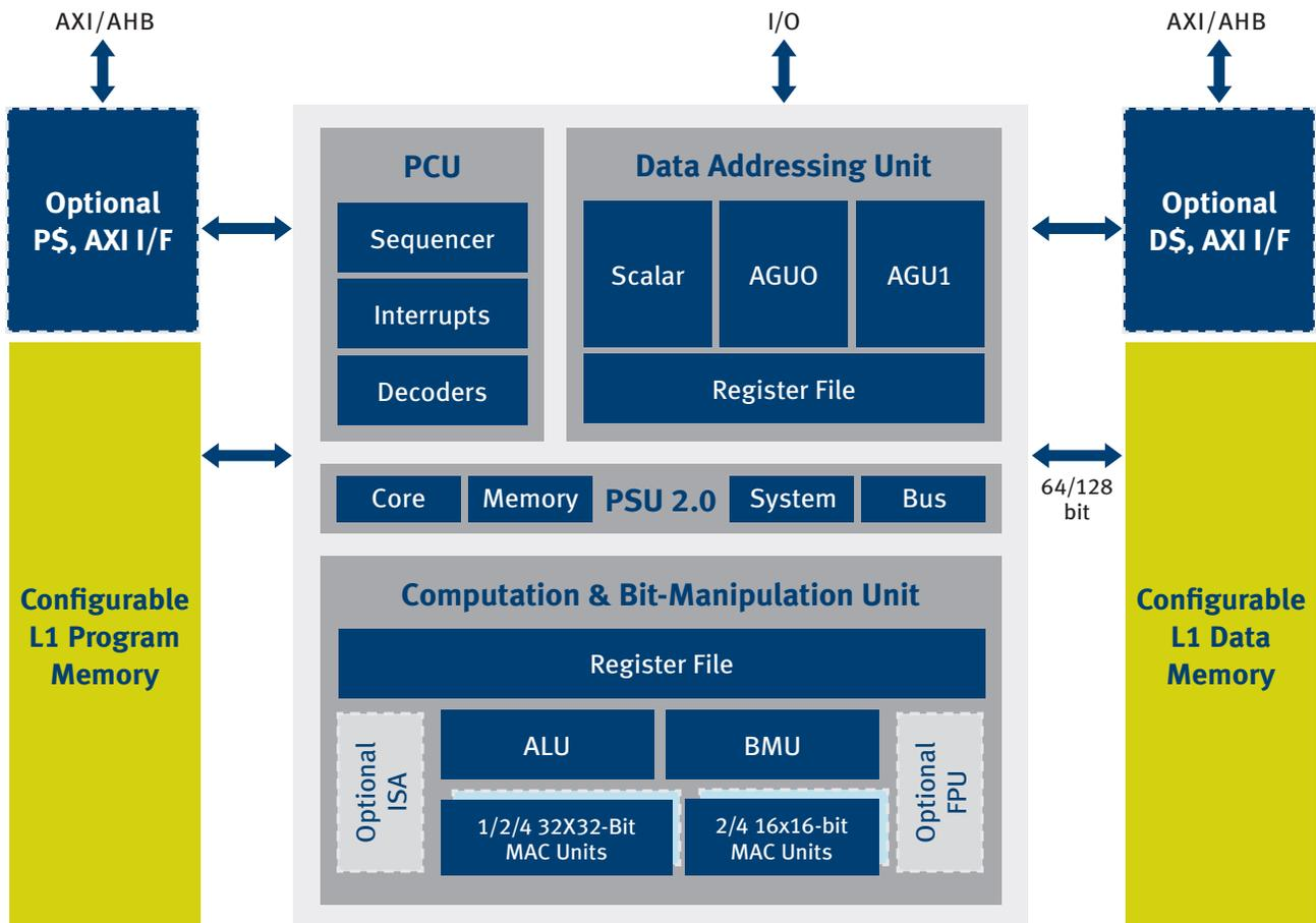
CEVA-TL410 with data and instruction cache controllers and a master/slave AXI system interface (the CEVA-TL421 augments the CEVA-TL411 with the same high-end capabilities). All CEVA-TeakLite-4 architecture-compliant cores are fully compatible with each other and with previous generation CEVA-TeakLite family cores.
