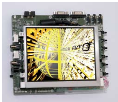
CEVA CDM development Board with LCD touch screen
