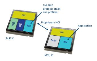
The CEVA RivieraWaves Bluetooth low energy software architecture is such that most of the components can be put in ROM, with GATT service database and profiles sitting in SRAM. This allows the implementation of low cost solution while maintaining full scalability and upgradability for future services/profiles support.
